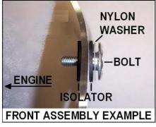
Place the one-piece front bracket onto the frame rails in its approximate location.
